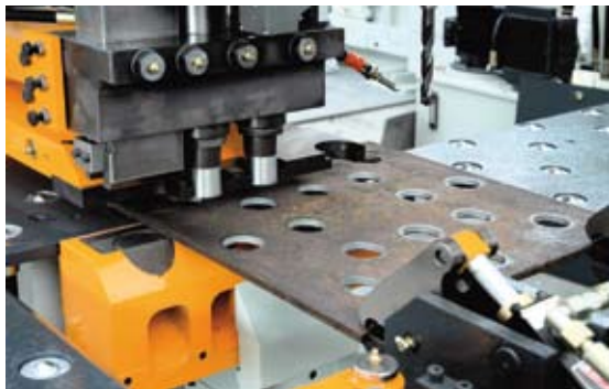
Drilling, punching and marking units
